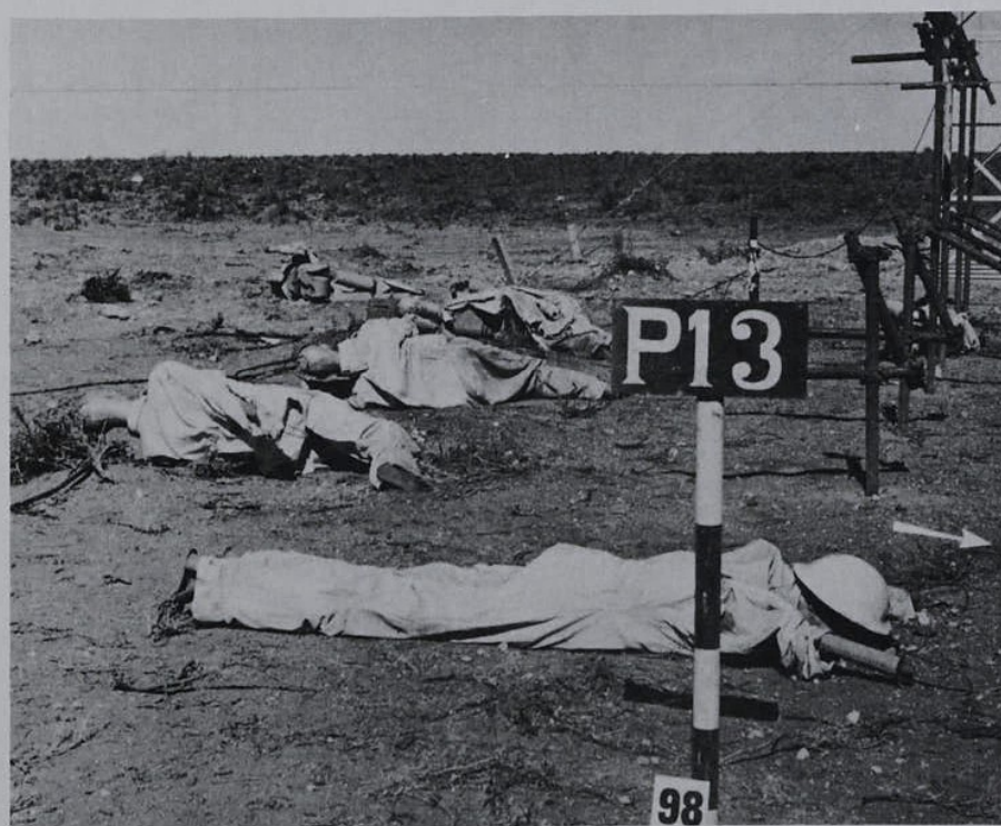
FIGURE 11. ROUND 2. DUMMIES AT 2390 ft AFTER FIRING. NOTE CAMERA TOWER IN BACKGROUND, AND LACK OF MOVEMENT OF THE PRONE FACING DUMMY
